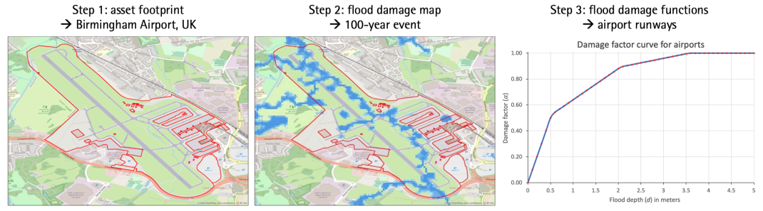
Figure 2: Baseline Flood Risk Metrics (100-year event), Birmingham Airport, UK
