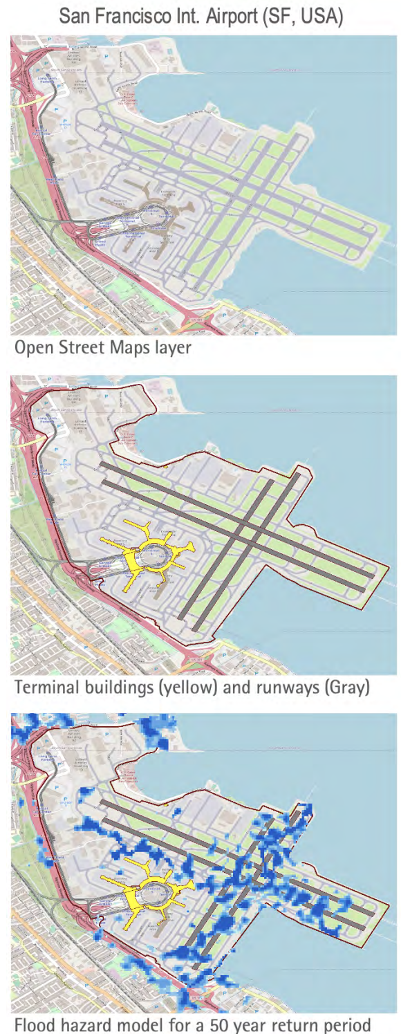
Figure 3: Example: airport's terminal and runways identification and flood model for a 50 year return period
